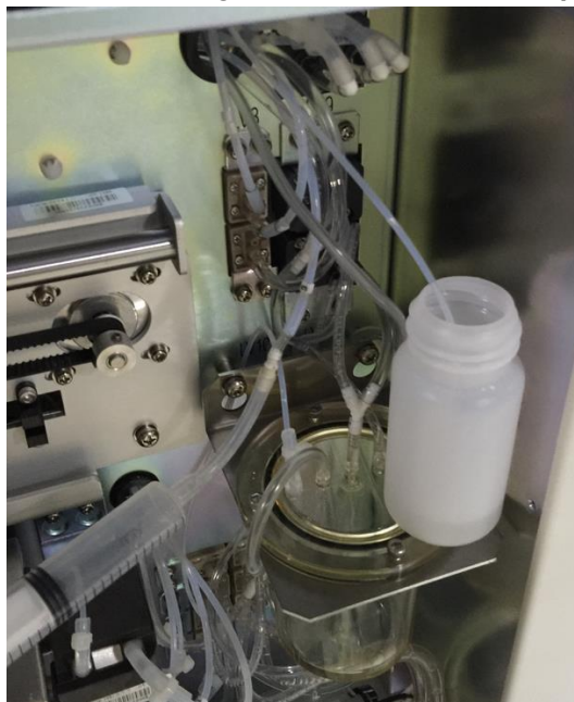
Figure 2-27 Cleaning the flow chamber/DIFF probe
