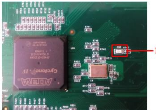
Figure 2-45 Indicator of FPGA working status
