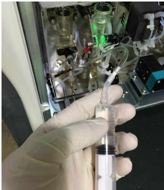
Figure 2-28 Cleaning the RBC-bath aperture
