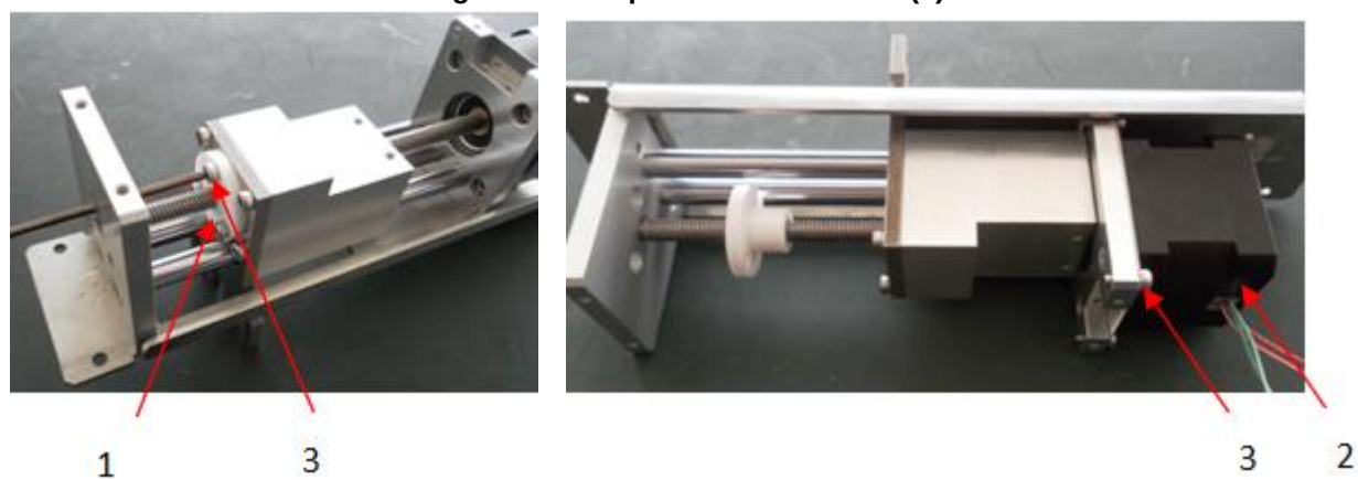
Figure 3-21 Replacement of motor (2)
